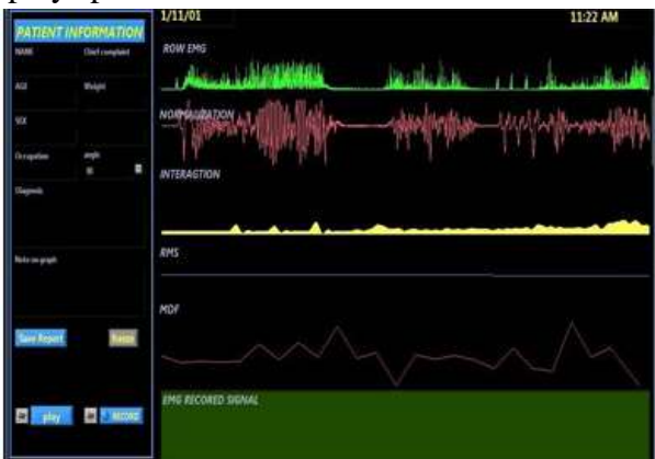
Fig 10: The GUI of the proposed Wireless EMG system with recorded and processed EMG data.
